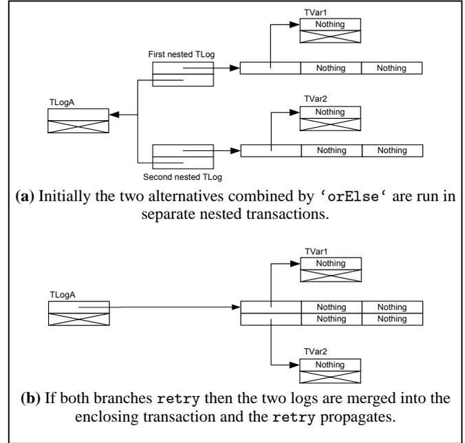
(a) Initially the two alternatives combined by ‘orElse’ are run in separate nested transactions.
